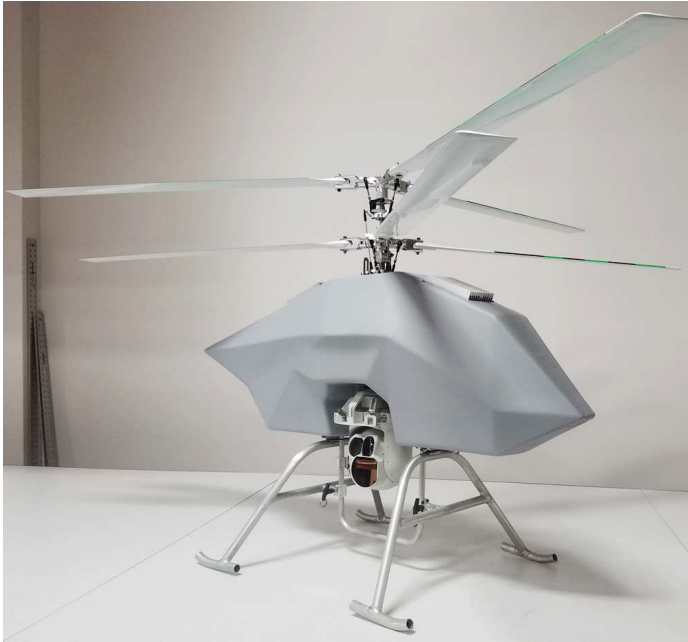
The tethered, coaxial-rotor Bolt can lift a 15-lb. gimballed payload to 800-ft. altitude. Credit: Drone Aviation Corp.
