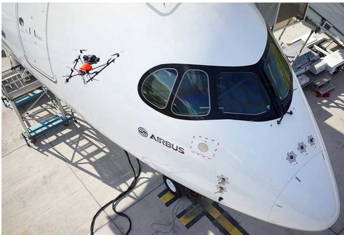
In Airbus tests, a small unmanned aircraft is used to inspect aircraft exterior quality. Credit: Airbus
