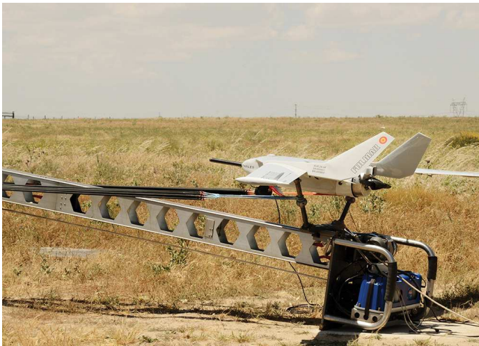
Flying-wing Fulmar X is designed for operation from confined spaces, such as ships. Credit: Thales
