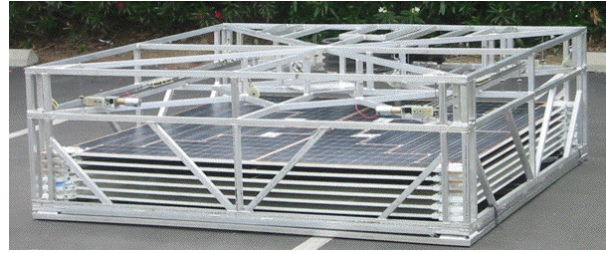
Figure 4 Solar Array Support Structure
