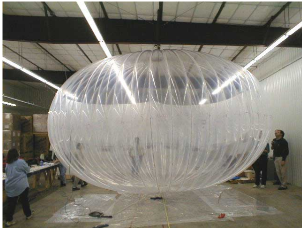
Fig. 2. ULDB Scale model Pumpkin Balloon Test (courtesy NASA Balloon Programs Office)
